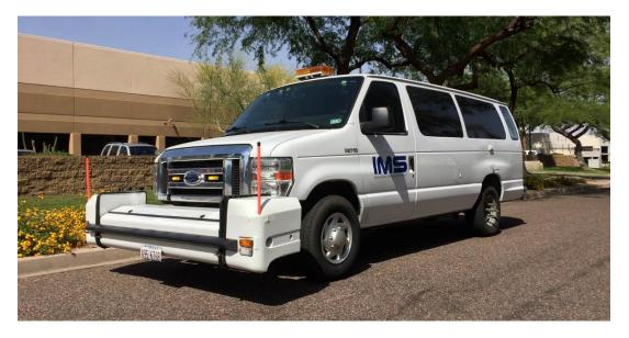
Figure 5 – Laser Road Surface Tester (Laser RST)
